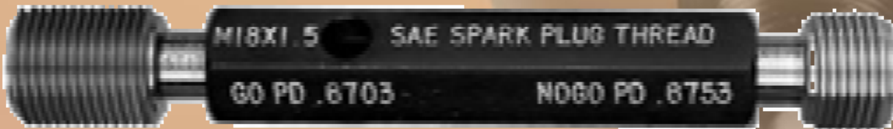
18mm x 1.5 SAE Spark Plug Thread Go / No-Go Gage
